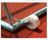
**110061:** The transport wheels for goal posts are made from polyamide. The wheels measure a diameter of 200 mm. The support structure is realized by aluminium. The wheels are mounted with stainless steel screws. The item is directly can be fixed to the goal post on site.
