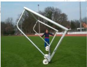
The counterweights are made from aluminium. The weights are fixed on the back side of the bar frame. The weights provide sufficient weight to prevent the goal from toppling over in accordance with the EN standard. The wheels for the counterweights are made from polyamide. They measure a diameter of 200 mm. The wheels are used to move the goal around comfortably.
