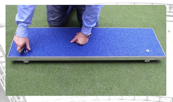
40011: The blanking beam made from aluminium with the dimensions  $122 \times 34 \times 10$  cm. This beam is not covered at the factory and can be covered on site. The dimension fits perfectly the installation trough and is equipped with stainless steel vertical adjustment bolts to level the blanking beams, and with horizontal ones to secure it to the installation trough, preventing it from moving during use.
