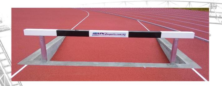
The water ditch hurdle is made from aluminium and a crossbar. There are two options for crossbars. Option 1 is a multi-layered laminated timber crossbar. Option 2 is a synthetic material one with an integrated aluminium core. The water ditch hurdle can be adjusted in height. The heights are 76.2 and 91.4 cm. The crossbar measures a total length of 3.66 m. The crossbar is a square 12.7 cm. The wood is painted with a special paint, which is long lasting even in a strong weather influence.
