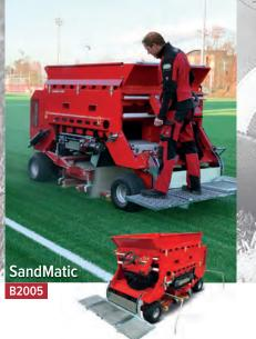
Ride-on machine for the filling of artificial turf.
