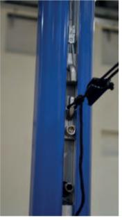
Volleyball competition posts made of oval anodised aluminium profiles. Our competition posts have a  $120 \times 100$  mm cross-section and a wall thickness of 4 to 6 mm. The net tensioning device and height adjustment mechanism are incorporated in the competition posts. The height can be easily and smoothly adjusted using a crank handle which can be removed during a game or for storage.
