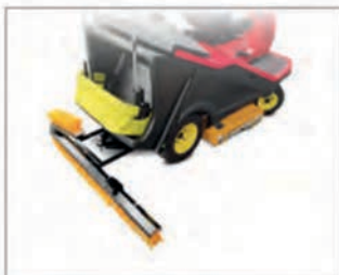
Expanded drag brush, working width 1.600 mm
