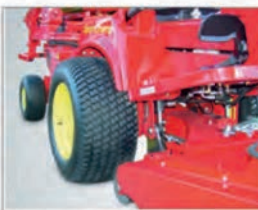
Tires especially for use on grassy surfaces ensure low pressure on the ground
