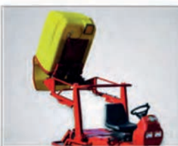
SC2D4HL: hydraulic high-level emptying up to 2.000 mm
