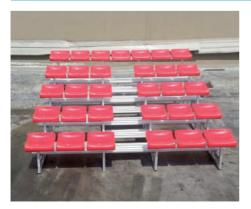
The five row bench 'Vindico II' with plastic seats and staircase is made of aluminium structure and plastic seats. The bench provides five rows of seating and has a total capacity of 31 seats. The bench measures a length of 3.1 m. The seats are made of UV protected plastic. The stairs are made from a special aluminium profile. The profiles are anodized and have an anti-slip surface. The system is dismantling and can be easily assembled at any site. **Order No. 139000**
