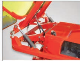
SC2D: Hydraulic lifting for tipping the filter box
