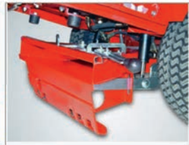
Practical coupling system for mounting all attachment without tools
