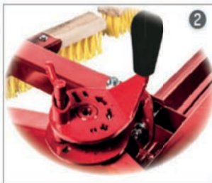
Adjustment spindle lock mechanism for Working depth
