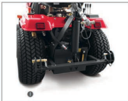
3-point rear attachment system
