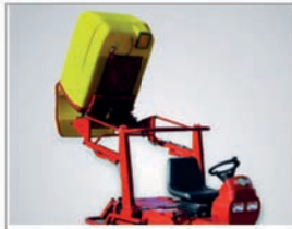
SC2D4HL: Hydraulic high-level emptying up to 2.000mm
