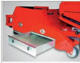
The vibrating screen separates dirt from the infill and spreads the infill on the artificial turf again at the same time
