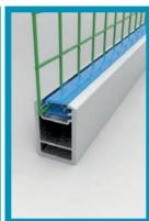
The 'flap down' net suspension system is a fully integrated and closed system. This means, all suspension parts are placed inside the goal post profile. The slot for the net suspension is covered to allow a smooth and safe appearance of the goal post.
